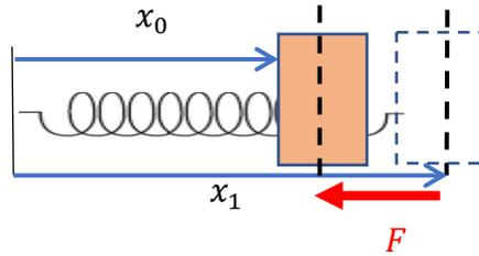
**Fig. 2** Single spring attached to a mass at one end. The dotted object is after the extension occurs.
