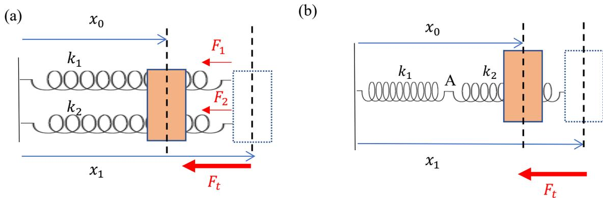
**Fig. 3:** Two spring systems that are in (a) parallel and (b) series. Only the extension of the system is shown where the dotted region is the object after extension.
